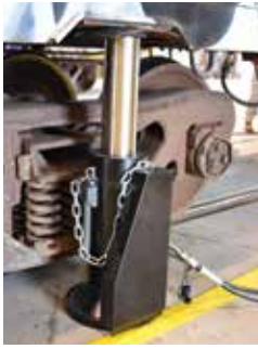
Rail Car Jack, JDR80, lifting the back of a rail car for the operator to start maintenance on the car's wheels.
